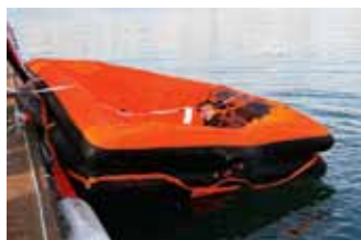
4 The tubes inflate first, then the canopy support fills with air...
