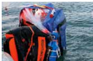
2 With the slack removed, a sharp tug on the painter line...
