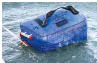
1 Throw the bag in the water and pull out the slack in the painter.
