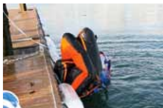
3 ...and the raft begins to inflate, bursting out of its bag.
