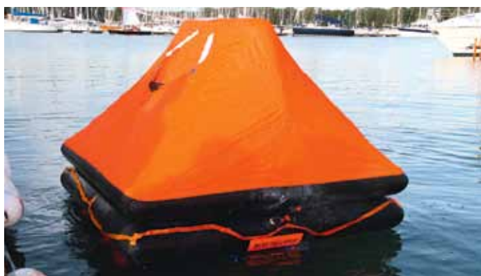
5 ...erecting the canopy. Over-pressure vents release any excess CO 2 . Some rafts have the sea anchor deploy automatically, while others store it internally, requiring manual deployment.
