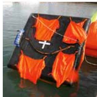
Good-sized ballast pockets gave the raft stability...
